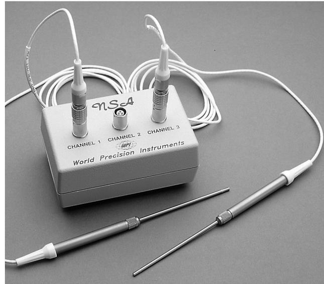
Electrochemical sensors require polarization prior to use. Polarization of this class of device serves two distinct purposes: it activates the electrocatalytic surface of the sensor to optimize performance; and it stabilizes the background current, allowing reliable measurement of signals.
